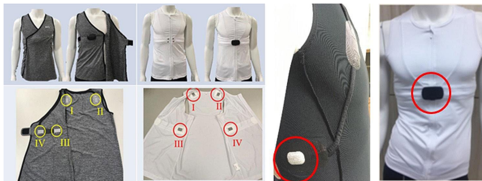
Fig. 1 Views of the smart vest with the four locations for the sensors: cervical spine, upper abdomen, body mass center, and both sides of the waist (I, II, III, and IV, respectively) The images on the far right show the conductive knitted fabric containing the buckle used to secure the vest and complete the circuit
