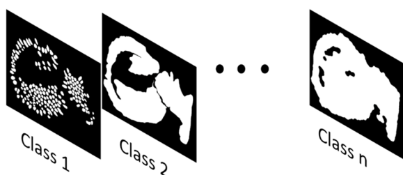
Fig. 3 Adaptable multichannel array format for multiple segmented annotation classes. MMIR allows the load of n number of classes using an array, the required array format is [x, y, nC] , where 'x' and 'y' correspond to the images dimensions, and 'nC' denotes the number of classes
